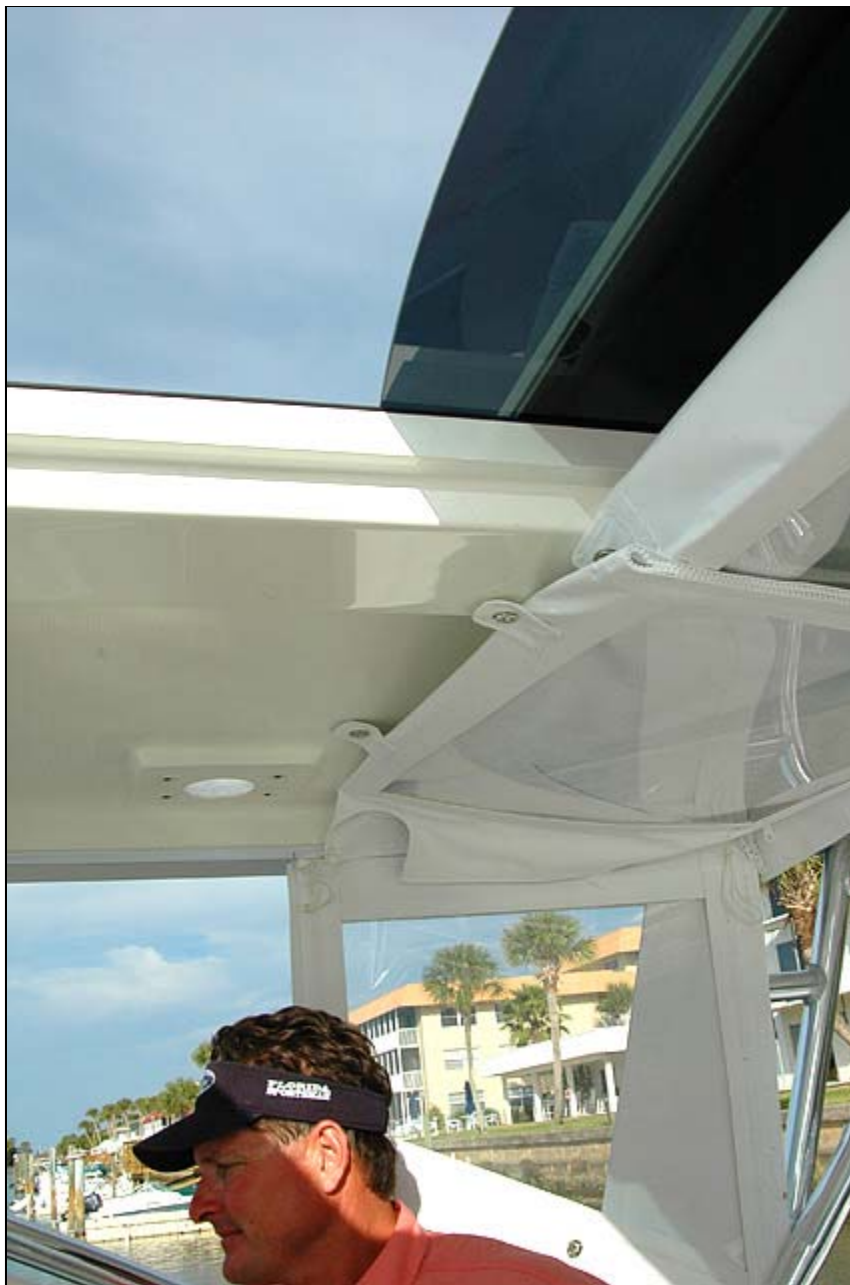
The sunroof lets the light in on the bridge.
