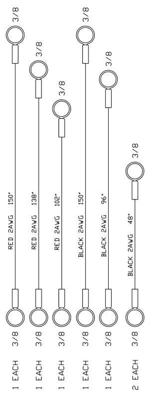
WIRING HARNESS - HULL
