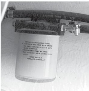
A fuel filter is installed in the transom area of your EdgeWater 260CC or 247CC. This is a fuel/water separator type of filter and is designed to prevent water from entering your engine. The fuel filter element is a spin-off type element. At a minimum, this element should be replaced at the beginning of every boating season. Always carry a filter wrench and spare filter of the type supplied on your boat.
