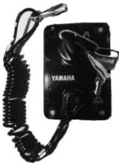
This device is designed to prevent the operator falling overboard while the engine remains running. The engine stop switch lanyard should always be worn by the operator, while the boat is in motion. Pulling the lanyard from the control will stop the engine. If the engine will not crank properly, the lanyard may not be properly attached to the engine stop switch.
