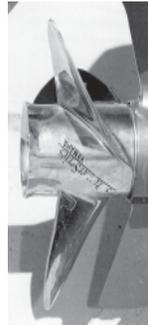
A turning propeller moves the boat through the water, forward or backward. They should always be clean and free from nicks or dings, which can adversely affect performance. Your dealer can assist you in the proper selection of a propeller for your boat. This selection is based on the horsepower of the engine and its relationship to the size and weight of the boat.
